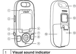
0 0 0 0 The visual sound indicator has two functions. One is to show the sound level detected by the baby unit. The other
